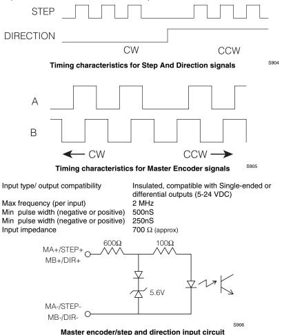
Differential signal inputs are preferred when using Step and Direction. Single ended inputs can be used but are not recommended. Sinking or sourcing outputs may also be connected to these inputs. The function of these inputs "Master Encoder" or "Step and Direction" is software selectable. Use MotionView set up program to choose desirable function.
