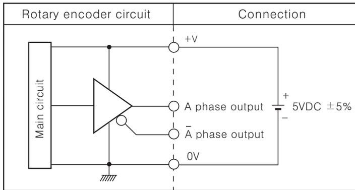
※All output circuit is the same A,  $\bar{A}$ , B,  $\bar{B}$ , Z,  $\bar{Z}$  phase.
