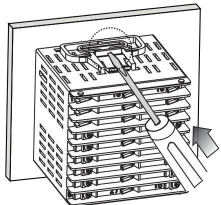
※ Insert product into a panel, fasten bracket by pushing with tools as shown above.
