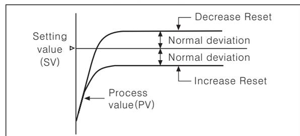
※Manual reset function is applicable only to P / PID control mode.
