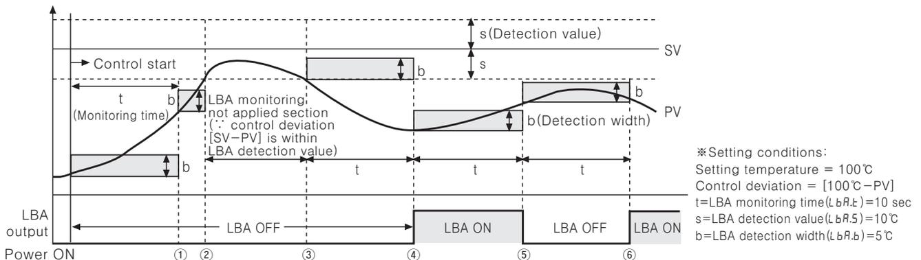
Control start ~ ①: LBA output OFF. As soon as power is supplied, control deviation [SV-PV] increases over LBA detection width (5°C) within LBA monitoring time (10sec).
