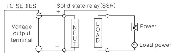
※SSR should be selected by the capacity of load, otherwise, it may short-circuit and result in a fire. Indirect heated should be used with SSR for efficient working.
