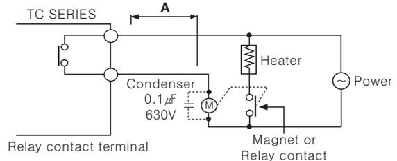
Keep power relay as far away as possible from temperature controller. If wires length of **A** is short, electromotive force occurred from a coil of magnet switch & power relay may flow in power line of the unit, it may cause malfunction. If wires length of **A** is short, please connect a mylar condenser 104 (630V) across coil of the power relay "M" to protect electromotive force.
