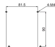
※Screw tightening torque for mounting: 1.8 to 2.5N·m
