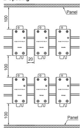
※When installing multiple SSRs, please keep space between SSRs for heat radiation. When installing SSRs horizontally (input part and output part on the same height), please supply less than 50% of the rated load current.
