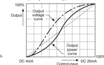
Controls phase angle which is proportional to control input (4-20mA) level.
