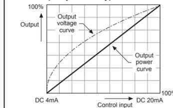
Controls output power which is proportional to control input (4-20mA) level.
