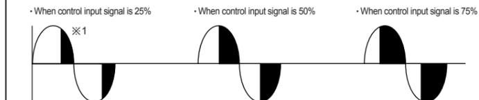
※1: The black parts of output waveform are output on the load.
