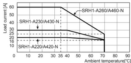
⚠ Since effectiveness of the heat radiation is decreased when multiple SSRs are installed closely, please supply less than 50% of the rated load current.
