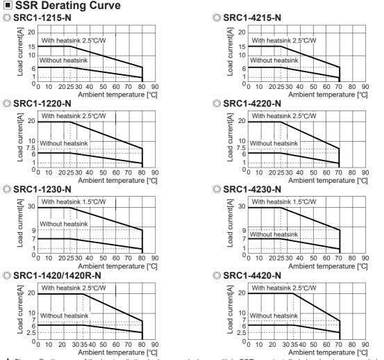
▲ Since effectiveness of the heat radiation is decreased when multiple SSRs are installed closely, please supply less than 50% of the rated load current.
