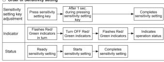
When pressing the sensitivity setting key below 1 sec., the sensitivity setting is canceled and it operates as the latest setting. If sensitivity is not enough or the setting is not correct, this unit may have malfunction.
