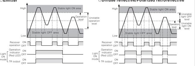
\*The waveform of 'Operation mode indicator' and 'TR output' is for Light ON mode, it is operated as reverse in Dark ON mode.
