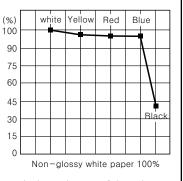
※It shows the rate of detecting distance by color of targets.
